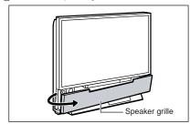
(2) Remove the lamp unit cover, loosening the screw fixing it. The screw is located on the left bottom.
